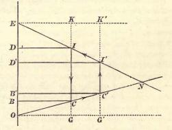
condition. And therefore the area B' B C C' will represent under the same condition the Thomson effect in the copper, D D' I' I that in the iron. Both of these represent absorption, for the current passes from cold to hot in copper, and from hot to cold in iron. It will be easily seen (by Euclid) that G C is the specific heat of electricity in copper at  $t^{\circ} C$ . (positive) while K I (negative) is that in iron.
